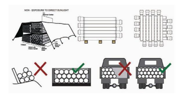
Unplasticized PVC pipes are strong but light, its specific gravity being approximately one-fifth of cast iron. As a result, these pipes are more easily handled than their metal counterparts. Reasonable care, however, should be exercised at all times and when off loading pipes should be lowered not dropped to the ground.
