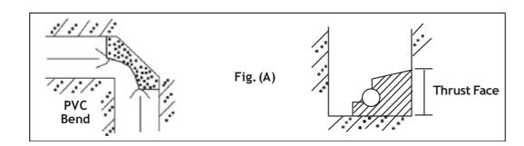
factor of 2.0 - 2.5 after a life of 50 years at maximum working pressure. In designing thrust blocks it is logical to apply a similar factor of safety after calculating thrust forces on the maximum foreseeable line pressure.
