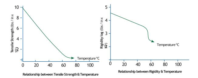
Where liquid carried in a pipeline is  $20^{\circ}$ C and the ambient temperature is  $20^{\circ}$ C - the maximum working pressure should be reduced by  $2^{\circ}$ 6 for every degree °C the fluid temperature is above  $20^{\circ}$ C. The aforementioned pressure reductions apply to maximum operating temperature of  $60^{\circ}$ C.
