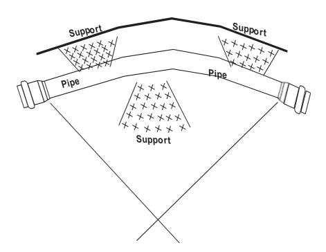
The ring integral socket permits an angular deflection at the joint of approx. 1.0 degree. The introduction of joint deflection is however, generally unnecessary flexible uPVC pipeline. Sufficient flexibility is provided by individual pipe lengths to enable gentle curves to be negotiated without imparting deflection at the joints.
