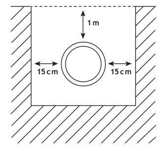
The width of trench for most purposes is enough to be 30 cm wider than the diameter of the pipe to allow enough room for jointing. Depth of cover should be at least 1 m from top of pipe to ground surface (it is wise to consider in early planning stages how future road widening plans could affect this depth of cover and to consider the frosting depth according to the local climate).
